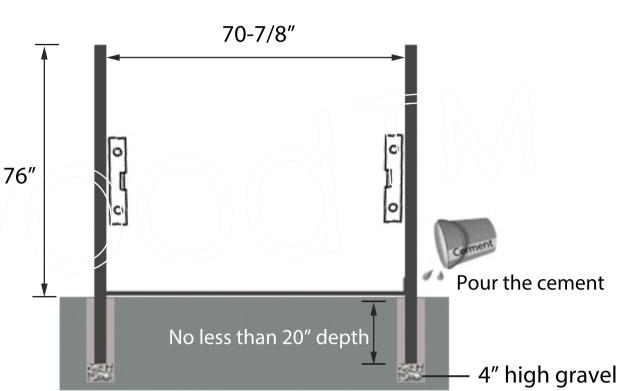
4, Pour the cement into the hole Double level the post Set aside untill cement dry
