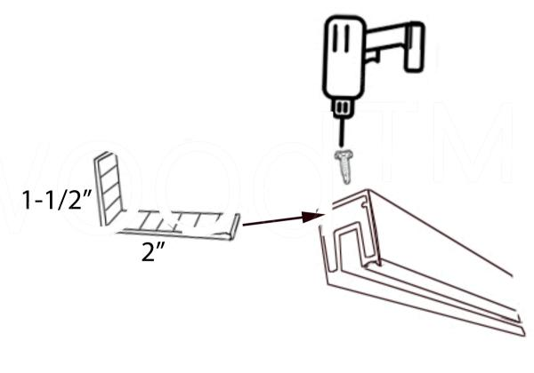
6, Insert L shape bracket into top rail channel Make sure insert the longer side (2") into the channel Secure the self tapping screw Repeat same assemble on the other side of top rail
